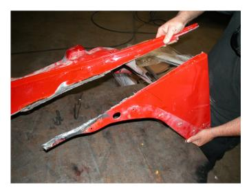
3.Remove the entire lower rear section as shown. Cut vertically down the inner side of the wheel well and remove all of the outside face of the fender.
