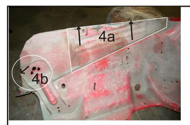
5. The fender is now ready to be re-installed on the Jeep. Clean up any sharp edges and apply some spray paint to any bare metal areas. Lay the new tube fender in place over top and bolt it back on in the factory mounting holes. Install the factory rubber hold down straps in the stock positions, and re-attach all factory components to their original positions.
